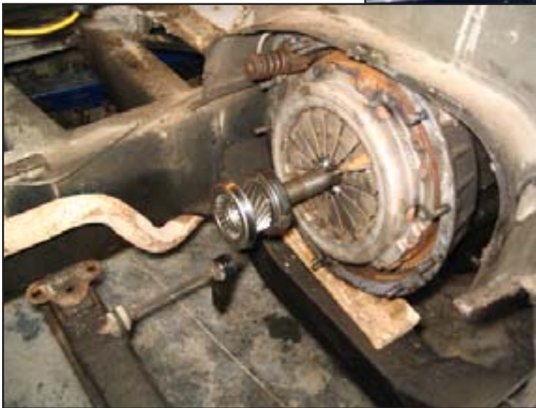
Fitting the new pressure plate on the clutch.
