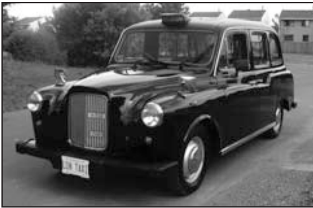
It's finally here, Murray's chariot of fire! Murr's 1988 FX4S Plus London Taxi with a 2.5 litre Land Rover diesel engine.
