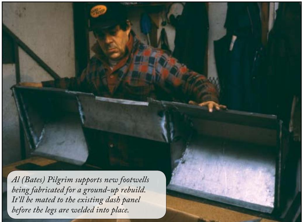
*Al (Bates) Pilgrim supports new footwells being fabricated for a ground-up rebuild. It'll be mated to the existing dash panel before the legs are welded into place.*
