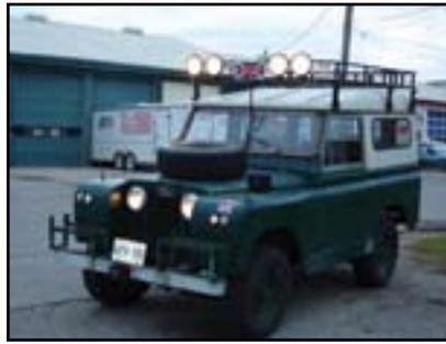
rust on the door bottoms and tops. The frame has been rebuilt and the bulkhead is in good shape. The wiring is a bit of a rats nest, the instrument panel has been cannibalized, and it leaks oil from all of the usual spots (some more than others) so there will be lots to keep me busy as I maintain and restore it.
