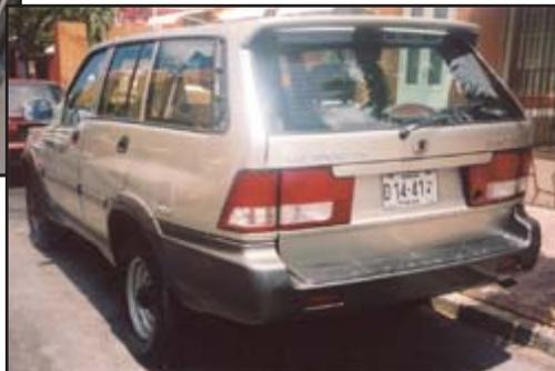
*Rear view of the Daewoo Muuso. Excessive overhang past rear axle hampers hill climbing but this vehicle manages fine on trails and on non-exacting off-roading.*
